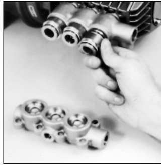
Figure 42: Removal of Adapter from Inlet Manifold
