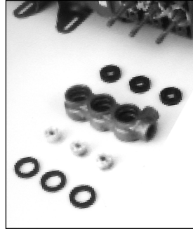
Figure 47: Plunger and Seals Arrangement
